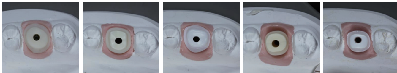
Fig. 2. Occlusal view of abutment samples on the respective master cast reveals differently pronounced emergence profiles and variously shaped abutment shoulders, despite mandatory abutment design (standardised wax-up of the abutment from try-in acrylic).
