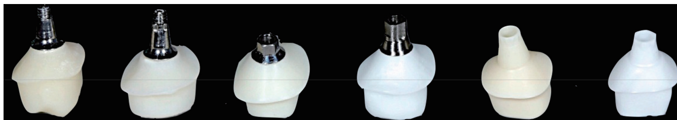
Fig. 1. The six one- and two-piece ceramic CAD/CAM abutments examined in the test and control group (left to right): Sample 1: Compartis (Dentsply Degudent, Hanau, Germany) CAD/CAM zirconia coping on titanium insert with implant-abutment connection for Ankylos C implant; Sample 2: Custom milled lithium- disilicate coping (IPS e.max, Ivoclar Vivadent GmbH, Liechtenstein) on titanium insert with implant-abutment connection for Ankylos C/X implant; Sample 3: Bego CADAbut (Bego Medical, Bremen, Germany): Zirconia coping on titanium insert with implant-abutment connection for Semados implant; Sample 4: MedentiCAD (Medentika Implant GmbH, Hügelsheim, Germany): Zirconia coping on titanium insert with implant-abutment connection for Straumann Bone Level implant; Sample 5: Atlantis (Dentsply Implants, Mannheim, Germany): Zirconia abutment including the implant-abutment connection for Astra OsseoSpeed implant; Sample 6: Procera (Nobel Biocare, Zürich, Switzerland): Zirconia abutment including the implant-abutment connection for Nobel Active implant.
