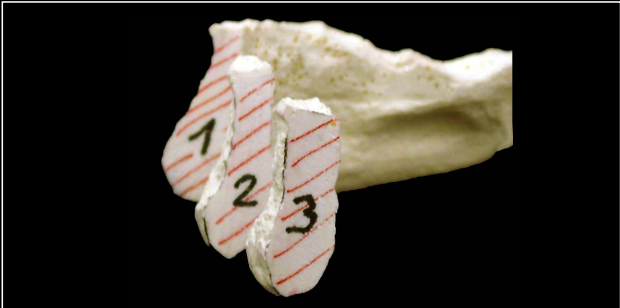
Sequential sectioning at 8 mm increments of sawbones
