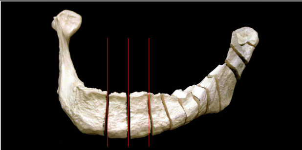
Sequential sectioning at 8 mm increments of sawbones
