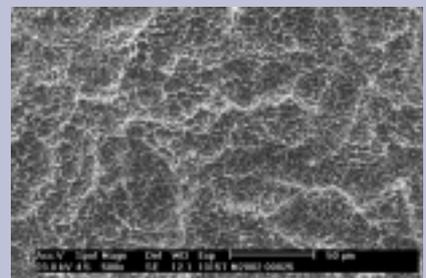
**Figure B2** Topography of grit-blasted and acid-etched surface.
