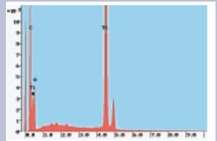
**Figure F5** XRM-analysis of embedded particle. Source: organic material.
