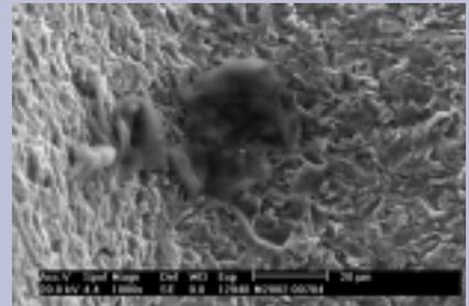
**Figure F4** Embedded particle; magnification 1000x.
