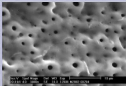
**Figure D3** Cracked surface and inhomogeneous distribution of porosities.
