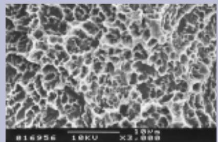
**Figure B3** Homogeneous topography of grit-blasted and acid-etched surface.
