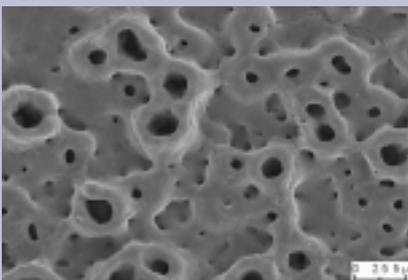
**Figure C3** Cracked surface and highly inhomogeneous distribution of porous structures.
