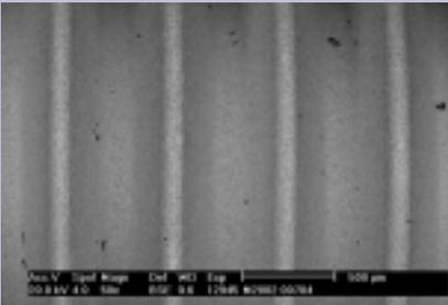
**Figure F1** Embedded particles on surface.
