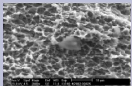
**Figure B4** Grit particle on surface; magnification 2000x.
