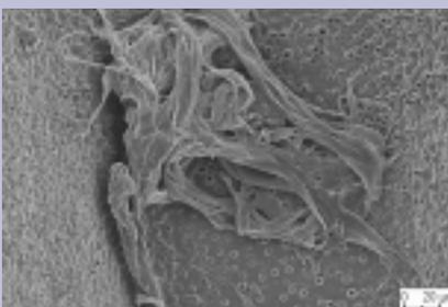
**Figure C4** Foreign fibrous particle on surface; magnification 500x.
